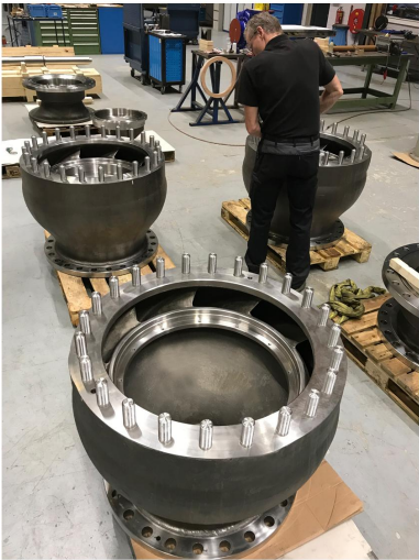
Assembly of 3 stage VS 1 diffuser bowls Below: Single stage VS1 pumps
