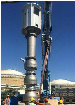
3 stage vertical turbine pump. (duplex)
