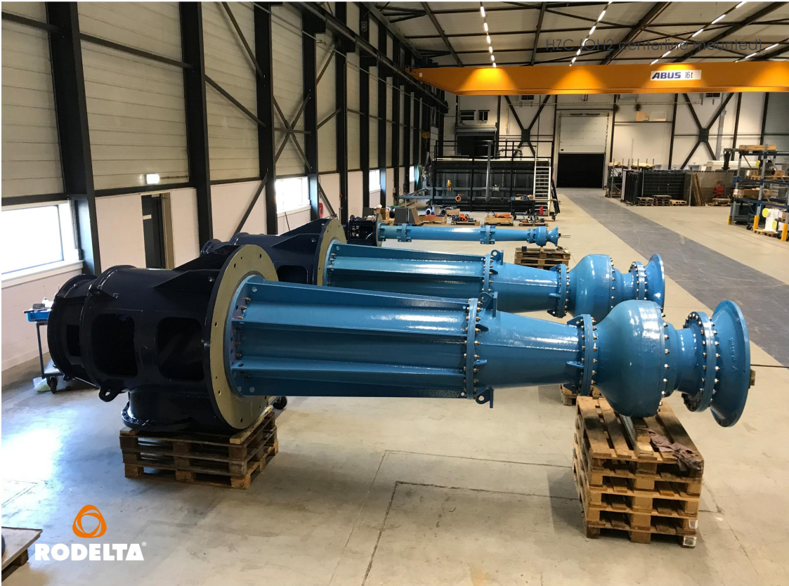
Assembly of 3 stage VS 1 diffuser bowls Below: Single stage VS1 pumps
