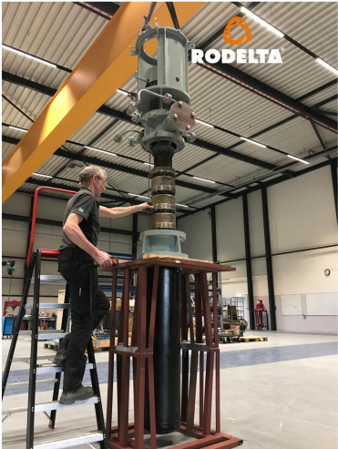
Below: Assembly VS6 pump
